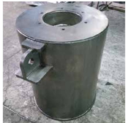
9" thick lead-poured lead lining
